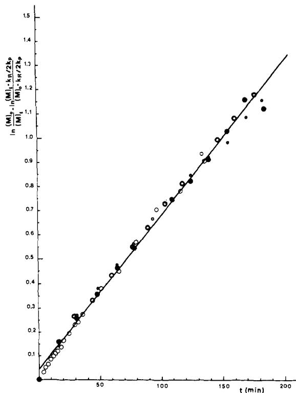
Figure 3. Fit of the kinetic data for the cyclization of sodium 8-bromooctanoate to a mixed first- and second-order treatment. The symbols are the same as for Figure 2.
