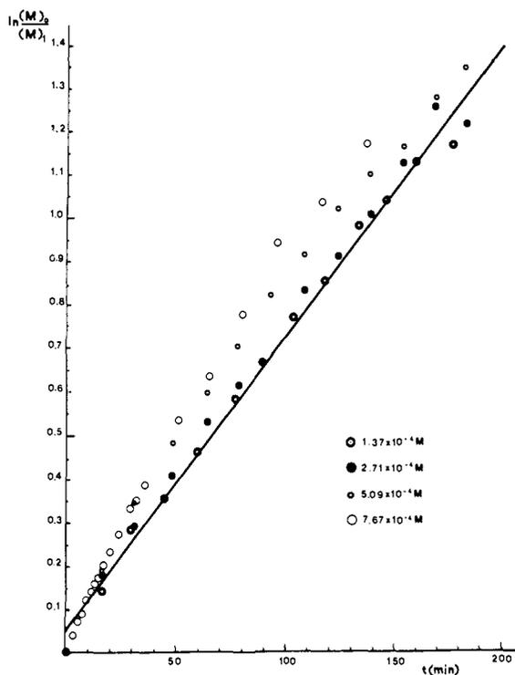
Figure 2. Deviations from a first-order kinetic correlation for the cyclization of sodium 8-bromooctanoate from four independent runs. Symbols refer to initial concentrations.
